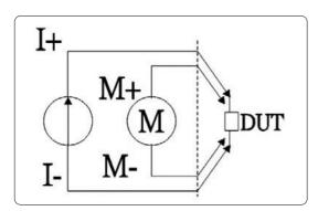
4-wire measurement, avoiding the resistance issues caused from adapting the fixture wires, low resistance of  $1m\Omega$ .
