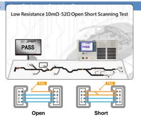
Low Resistance Test: Detect the open/short problem on the contact point of the terminal.
