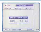
The Intermittence test function is swing test. Setting test time in seconds, the cable tester will continuously scan within the set time to perform a short-circuit judgment test.
