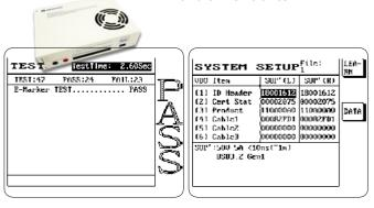
Learning test the USB Type-C E-Marker IC's code Reading E-Marker's VDO Data using the FX-000C28.
